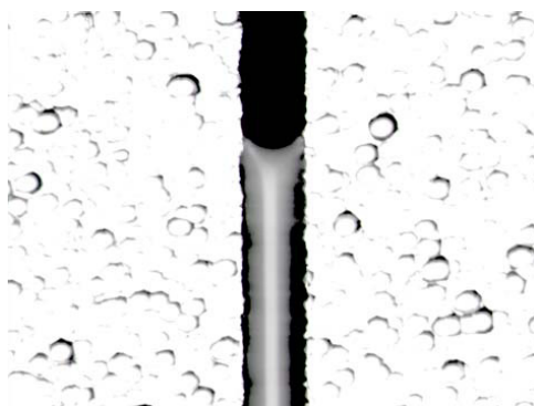
Figure 5. A 50:50 vol.:vol. MeOH:H 2 O mixture in a micro-machined capillary slot having a width w of 140 \mu\text{m} and a height h of 230 \mu\text{m} ( R = 1.64 ).
